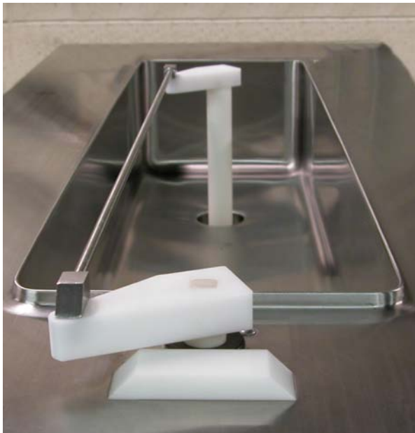
Figure 3-3 Flow Control Assembly
